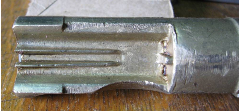
Original cast bronze STEN bolt:
