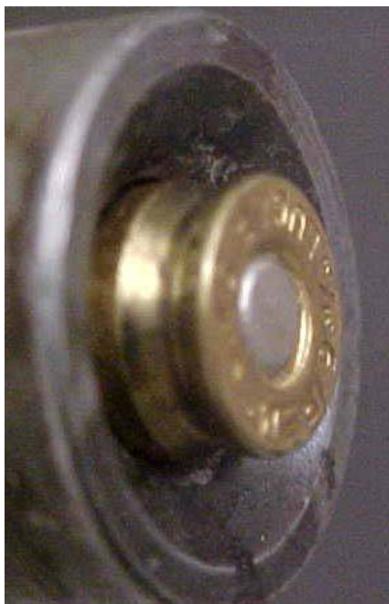
Original STEN chamber feed entrance:
