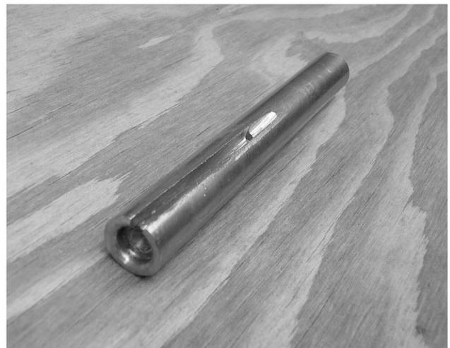
*The builder may choose to leave out the ejector and ejector slot in the bolt and hold the weapon with the magazine positioned to the left of the user, ejection port facing down.*
