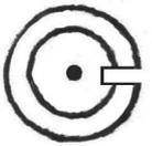
Cut 45mm long, 5mm deep slot along one side of the bolt body. This can be achieved using a combination of drilling and grinding using a 1mm slitting disc.
